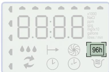
96 Hour Mode - With 96 hour mode on, the unit will never go more than 4 days between regenerations. More frequent regenerations help keep iron build up from occurring. This setting is recommended to be used when iron is present in your water supply.
