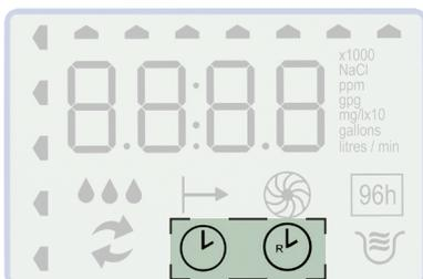
The clock icon will display when setting the time of day. The clock icon with an "R" on it will display when setting the regeneration time of day.
