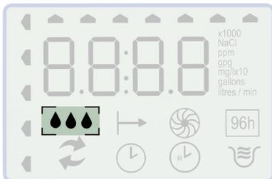
Indicates that water is flowing through the appliance; the water flow indicator animates whenever water is being used; useful for checking for proper plumbing and leaks.
