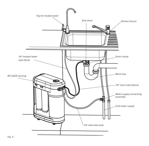
Find a convenient location for your RO-202S and the treated water tap. Attention should paid to prevent the supply tubes from bending and twisting (Fig. 3).
