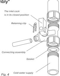
ATTENTION! The end of the pipeline must be flat, where the connecting assembly is connected. Do not use excessive force when tightening the clamping nut. Otherwise, it will damage the gasket.
