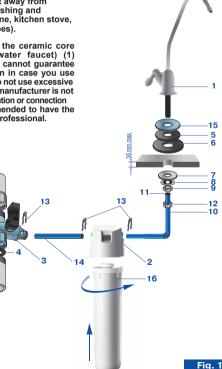
Warning! Don't apply any excessive force for the screw-tightening while connecting the shut off valve.
